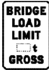
Bridge load limit (gross mass) sign
