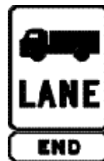
End truck lane sign
