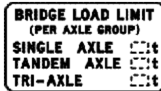
Bridge load limit (mass per axle group) sign
